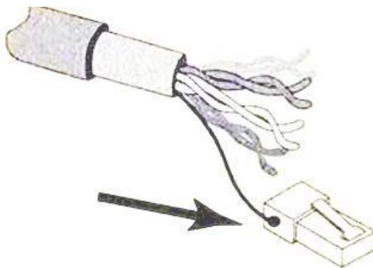
Grounding the STP shield cable (as shown below) , and make sure the metal RJ45 connector is tight shield.
