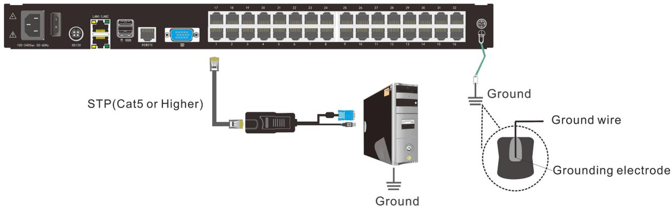
To improve the device safety, please make sure the device is connected to the ground and use the STP cable to connect the device. The STP cable contains four shielded twisted pair and one ground wire, the ground wire should be welded into the RJ-45 connector.
