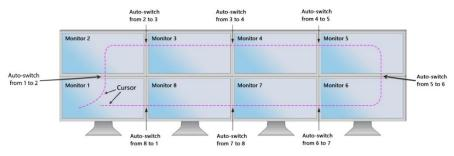
KM0108 automatically switches when the mouse moves between screens.
