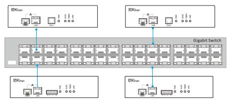
Configuration requirements: The electrical port of the network switch must reach a gigabit rate and support IGMP multicast.
